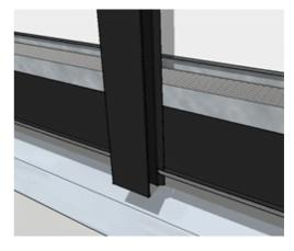
Where the Aluminum Joint Trim meets the Starter Strip , the Starter Strip should be cut 25mm from the lip to allow the Aluminum Joint Trim to descend 15mm below the Starter Strip. For the corner trim, the Starter Strip is cut 50mm.
